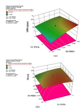
Fig.6 3-D graph (a) MRR (b) SR(surface roughness) [16]
