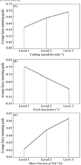
**Fig 8.**Response Graph for different level of machining parameters: (a)Cutting Speed; (b)Feed Rate; (c)MassFraction of SiC-Gr [15].
