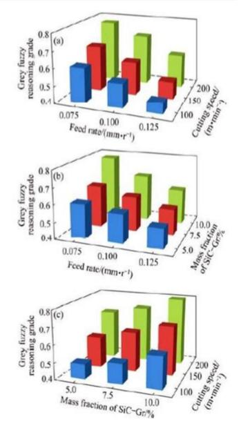
**Fig.9** Effect of Grey-fuzzy reasoning gradeon machining parameters: (a) feed rate and cutting speed
